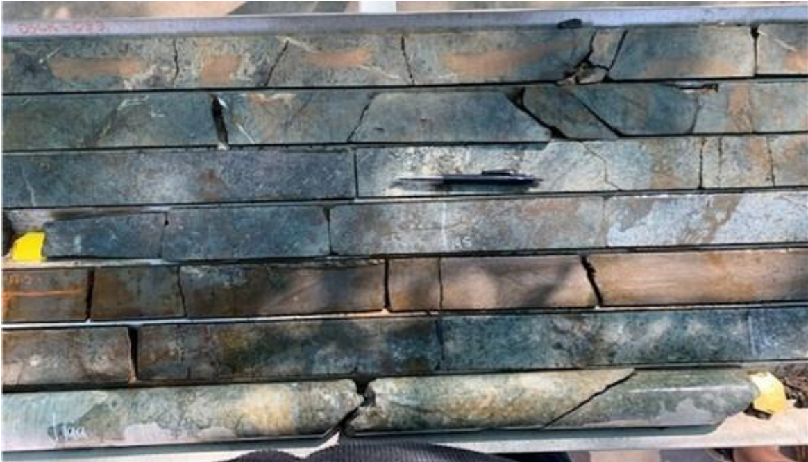
Figure 12-4: Mineralized Taxitic Gabbro with Massive Sulphides (BH083: 192 – 197 m)
