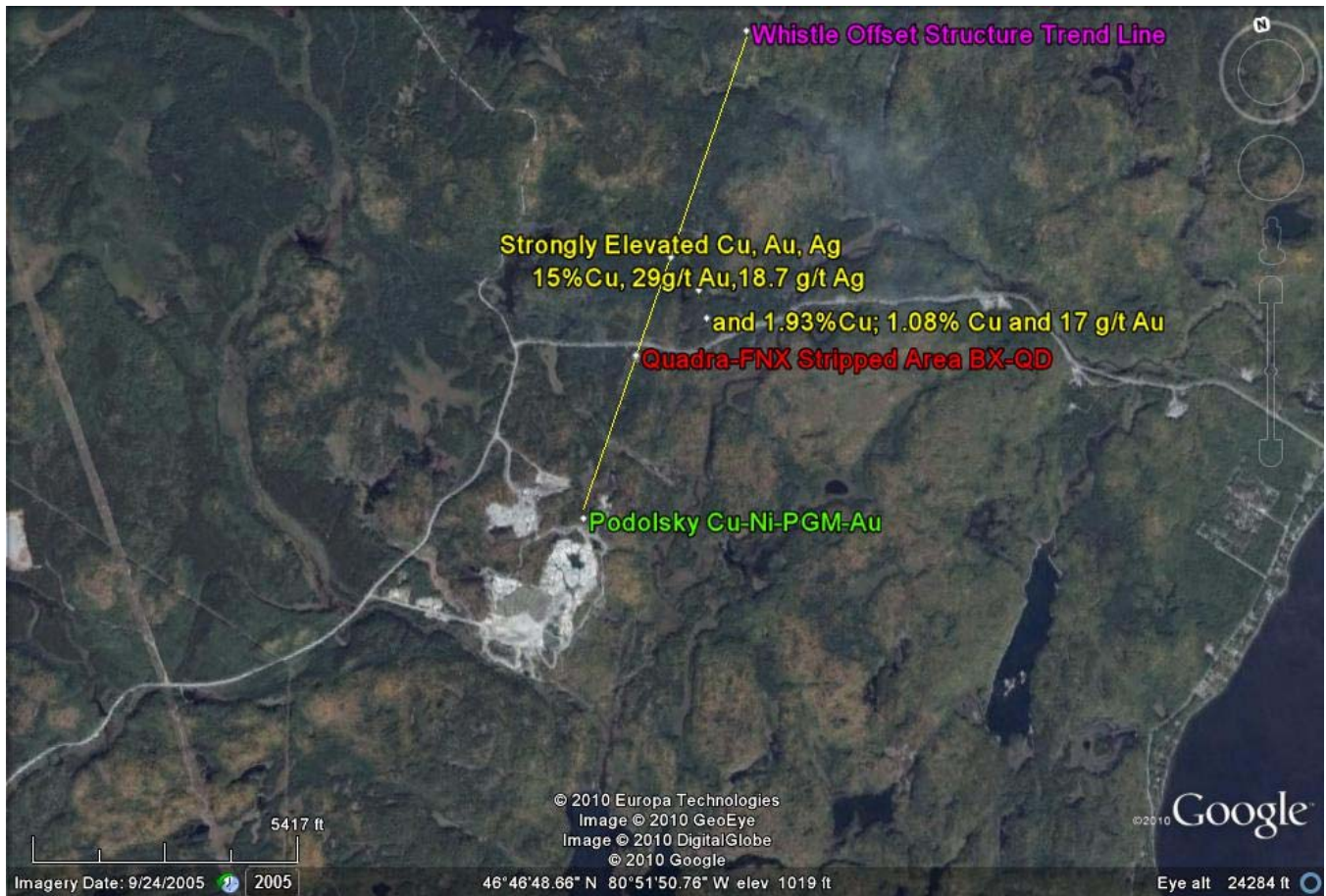
Figure 11. Google Earth image of the Whistle Offset trend line, Podolsky Cu-Au-Ni-PGM mine and strongly elevated Cu, Au and Ag assays, Post Creek property. Note: BX-QD refers to Sudbury breccias and volumetrically minor quartz diorite.
